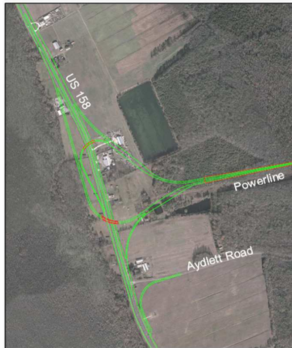
Compressed Y Interchange Design
